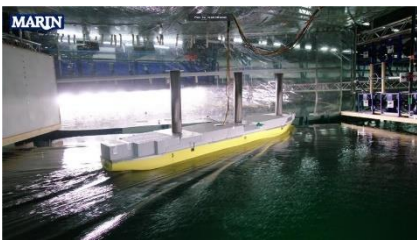
Model test in our Seakeeping and Manoeuvring Basin.
